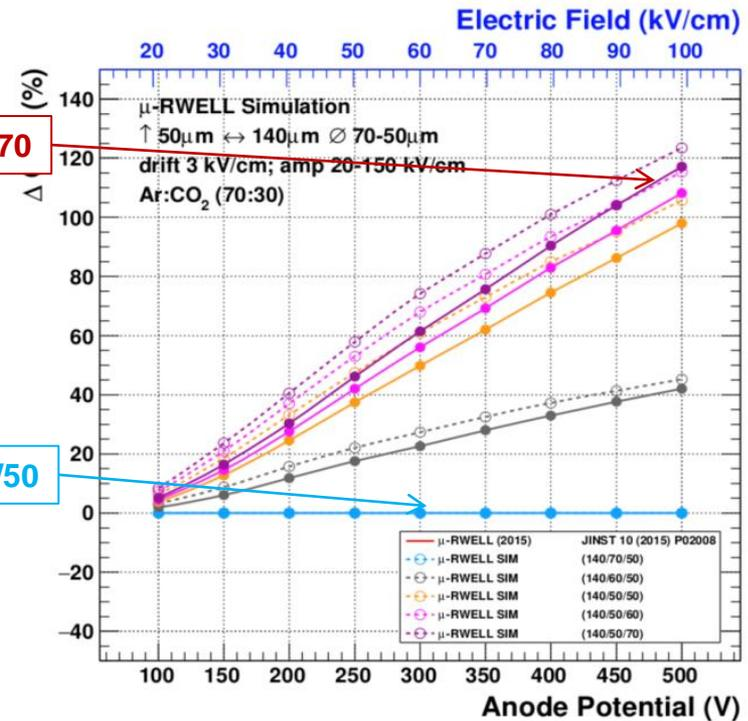
(b)  $\Delta G = (G_{\text{FTM}} - G_{\mu\text{-RWELL}})/G_{\mu\text{-RWELL}}$
