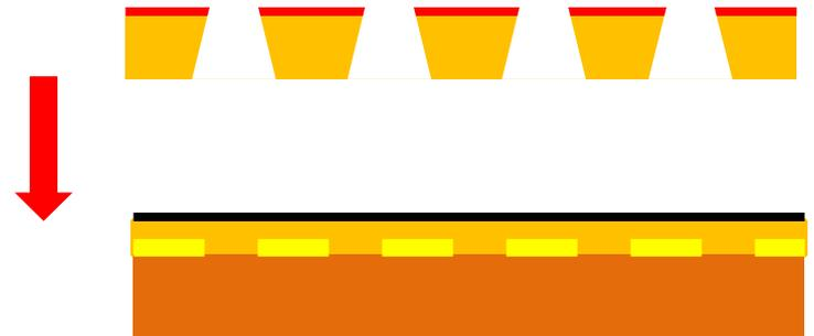
readout PCB with DLC-ed kapton foil embedded on top
