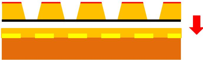
readout PCB is directly coupled with the amplification stage before the kapton etching
