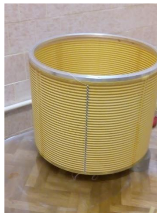
Figure 3. Field cage for the TPC prototype.
