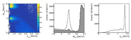
• A PID system with  $\pi/K$  separation up to about 1.45 GeV/c is necessary for amplitude analyses of the  $J/\psi$  decays.
