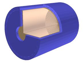
Only ASHIPH system has realistic geometry. The drift chamber is represented by a cylinder filled with air, outer detectors (calorimeter, muon system) are not implemented yet.
