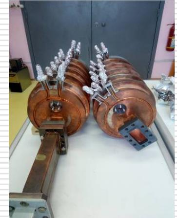
Prototype of the klystron
