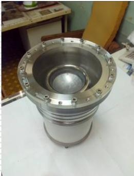
Vacuum waveguide window
