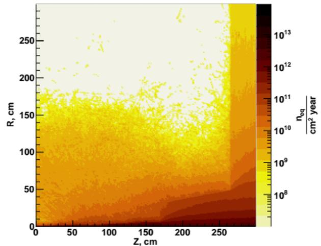
1 MeV equivalent neutron dose for silicon
