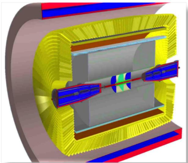
Detector geometry in DD4HEP
