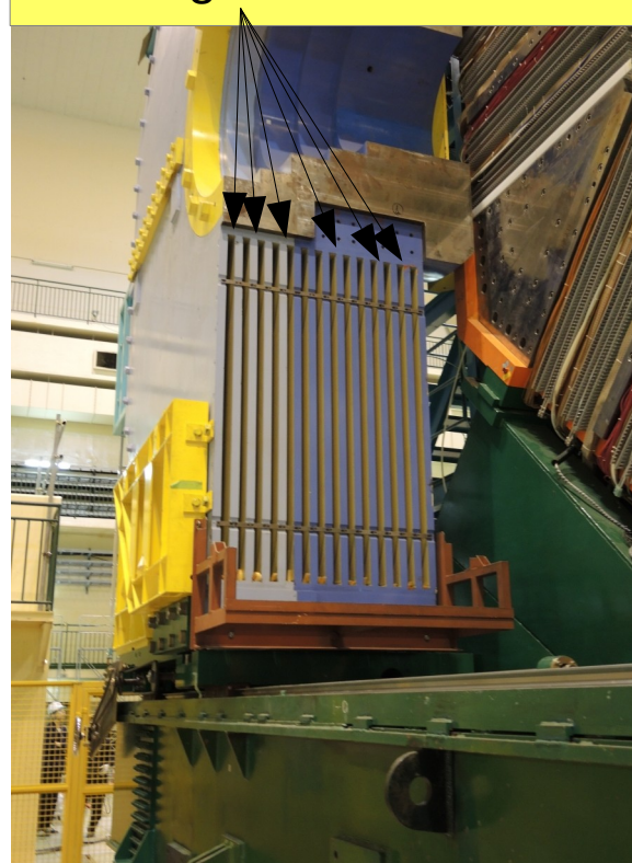
Installation gaps in the magnet flux return
