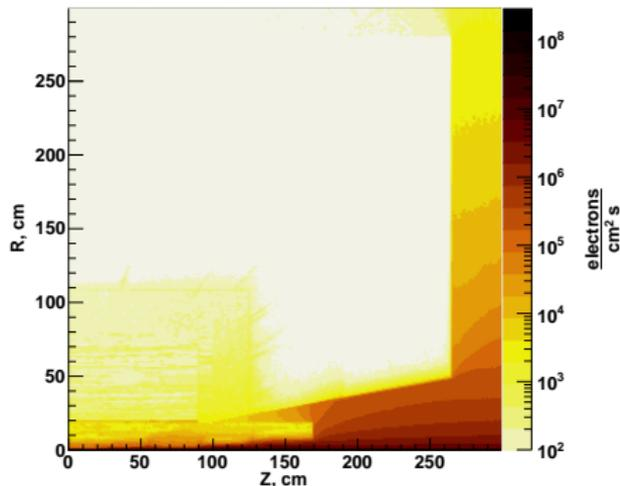
1 MeV equivalent neutron dose for silicon
