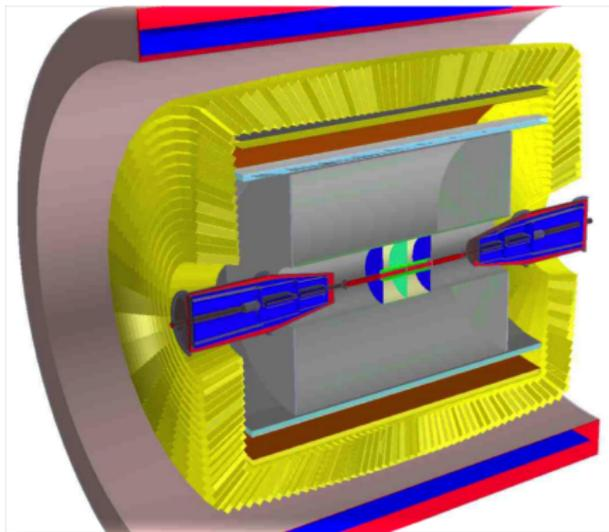
Detector geometry in DD4HEP
