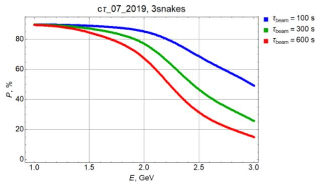
Dependence of beam polarization degree on energy for different time of beam doping
