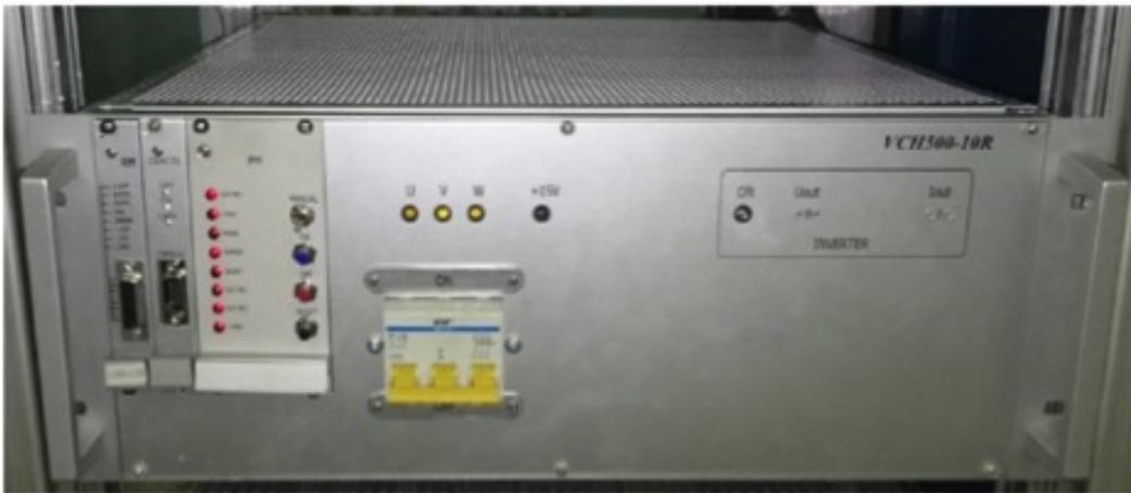
Figure 1.96. Appearance of current source VCH500-10-2Q.
