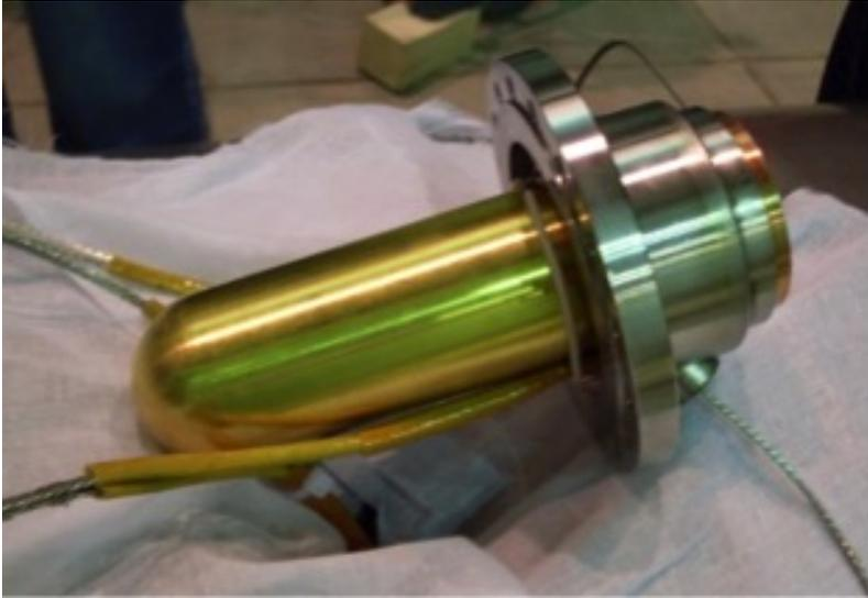
Figure 1.91. Appearance of gold-plated copper heat exchanger.
