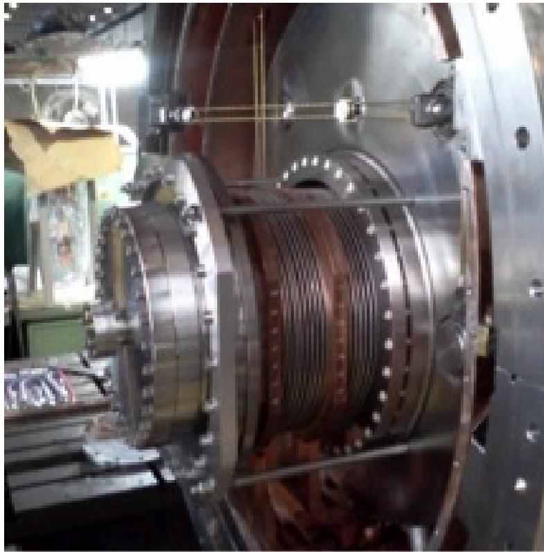
Figure 1.94. Appearance of output flange for connection with storage ring.
