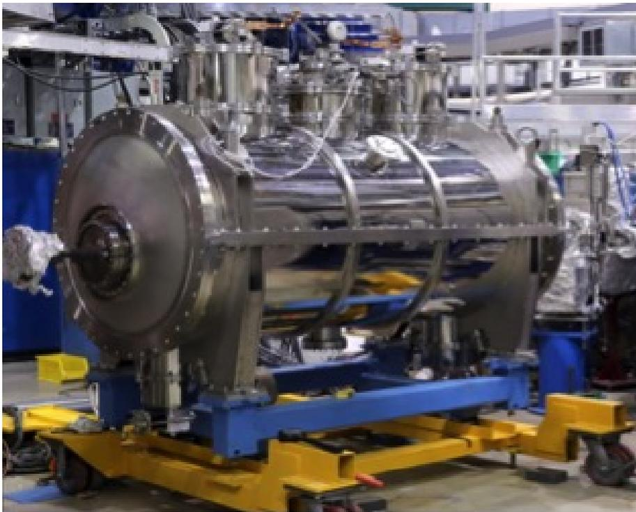
Figure 1.77. Appearance of cryostat of superconducting damping wiggler.
