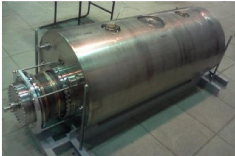
Figure 1.86. Helium vessel assembly.
