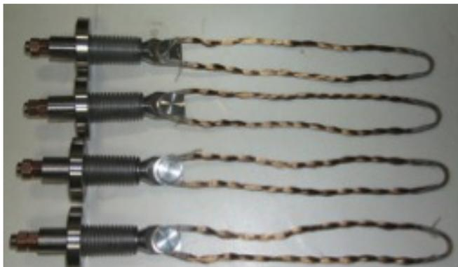
Figure 1.87. External view of adjustment assemblies and Kevlar suspensions.
